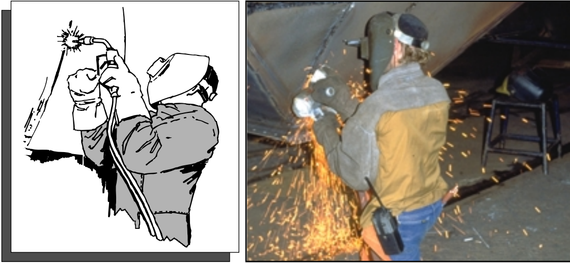
Fig. 1-9. Cape and bib for overhead and eye-level welding
