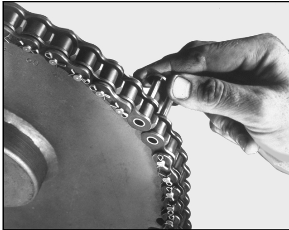
Fig. 1-9. Inserting connecting link in chain ends
