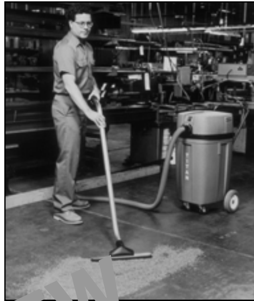
Fig. 1-9. Using vacuum to clean hard-surface floor
