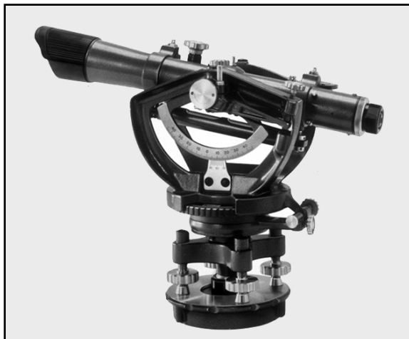
Fig. 1-3. Transit level for laying out building lines
