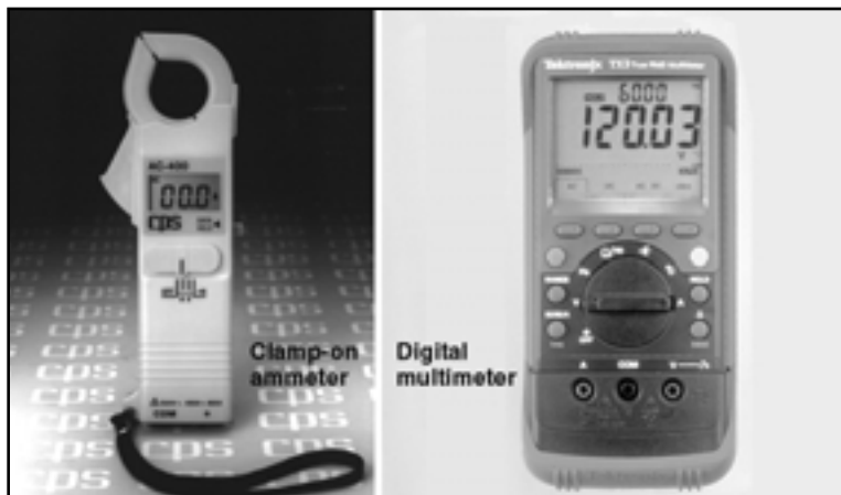
Fig. 1-5. Electrical test instruments
