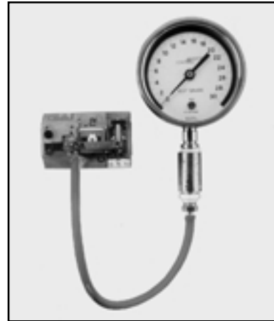
Fig. 1-6. Pressure gauge for calibrating pneumatic controls
