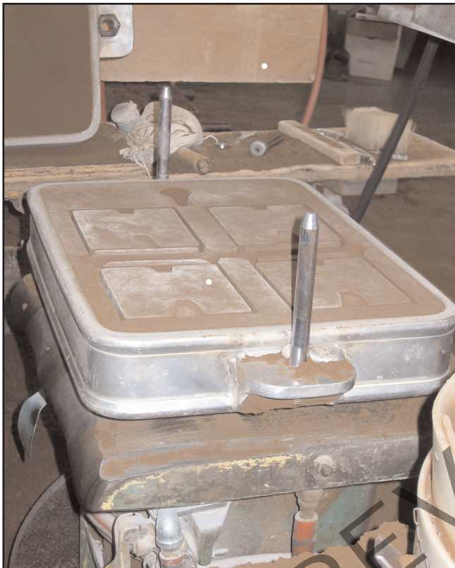
Fig. 1-9. A mold prepared for casting
