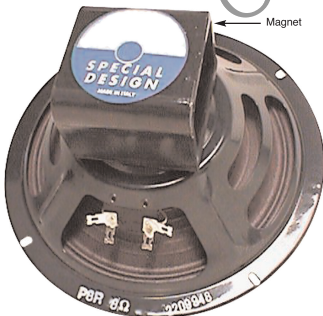
Fig. 1-1. Alnico magnet in a radio speaker
